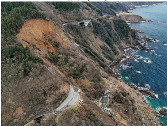
Road cut off due to slope failures Source: Kyodo News
