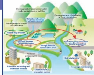
Basin flood control concept
